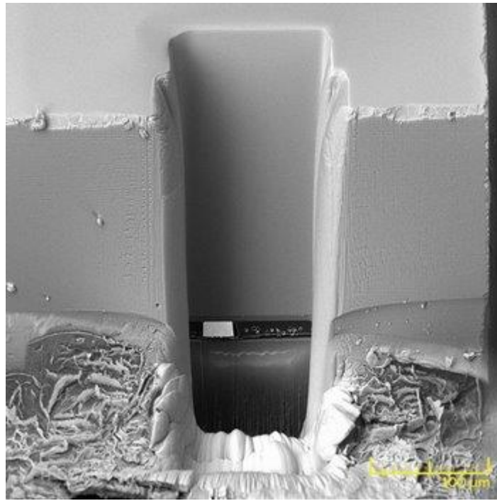
Fig. 2 Cross-section of integrated circuit made using Xe-PFIB technology
