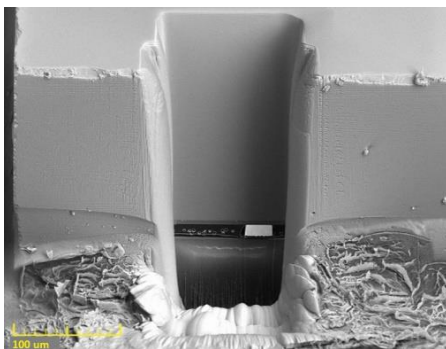
Large scale backside milling of TFT panel performed on Plasma FIB [exemplary image]
